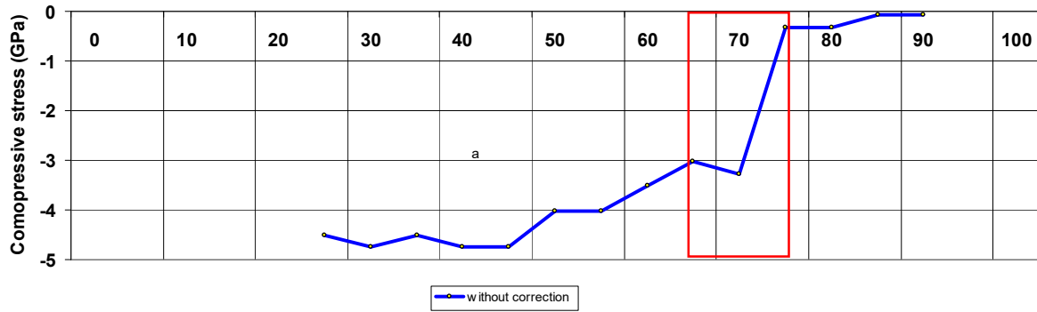
Fig. 5 – Recalculated compressive stresses in the nitriding layer \alpha' -Fe(N), N=0-5,7 wt%
